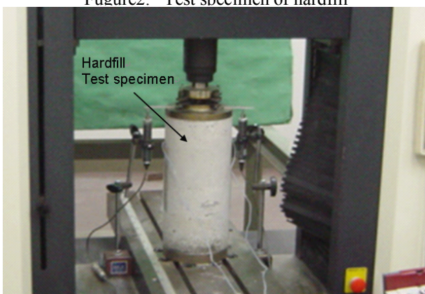
Figure3. Uniaxial compression test of hardfill Table 1 summarizes the test cases of cyclic loading tests.
